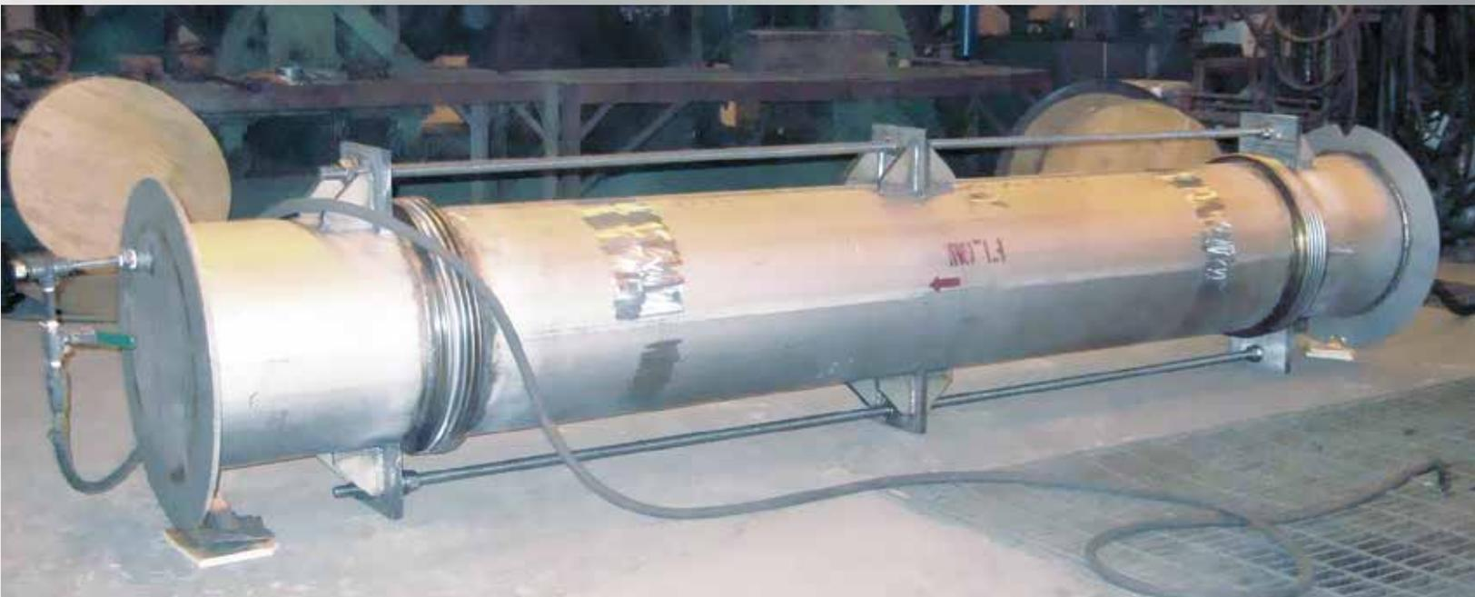
*Hydrostatic testing of a universal expansion joint*
