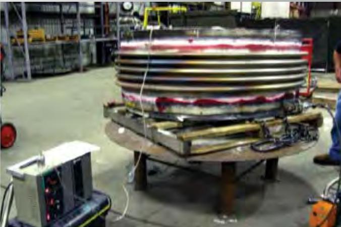
*Non-destructive testing such as dye penetrant inspection is regularly performed to check for cracks in the welds*
