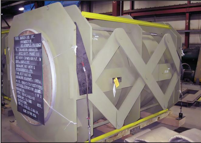
From complex expansion joints for the most severe service such as this assembly for a refinery FCC unit to simple single bellows seals for HRSG boilers, Badger supports almost any application
