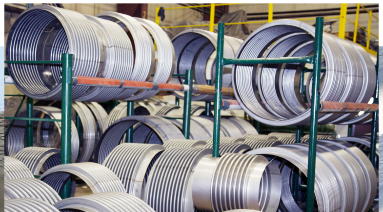
The selection of bellows material is one of the most important factors to consider in designing an expansion joint
