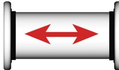
*Shown here, pressure thrust is restrained by the strength of the pipe between the blind flange attachments*
