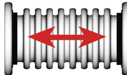
*When blind flanges are attached to the ends of unrestrained metal bellows, the bellows response to pressure thrust results in the bellows convolutions stretching out until it returns to its original tube form.*
