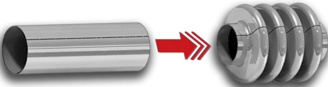
*After material selection, the bellows material is sheared and rolled into a tube, welded, and planished (as shown on the left). The tube is then processed on a bellows forming machine to add the convolutions as shown on the right.*
