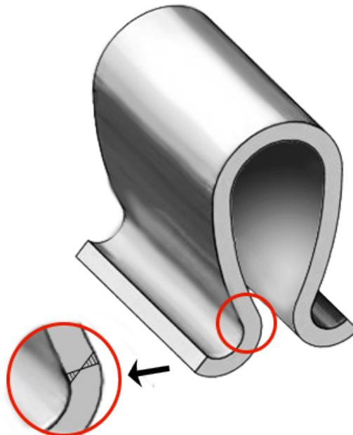
Metal bellows movements are normally designed to operate in the plastic range of materials and therefore will take a permanent “set” at the bellows rated movements. When a bellows compresses, extends, or angulates, the movement is absorbed by deformation of the sidewalls of the bellows convolutions. The stress caused by the sidewall deformation is defined as the “deflection bending stress, EJMA S6”. This stress is highest at the “root” and “crest” of the convolution.
