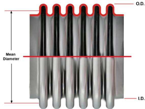
Pressure thrust forces are typically higher than all other system forces and are usually restrained by system anchors. If anchoring is insufficient or absent, bellows pressure thrust forces can also be restrained by externally-attached hardware such as Tie Rods, Hinges, or Gimbals.
